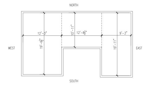
If you have a complex or odd shaped room, divide the room into sections (making blocks) and measure width and length.
